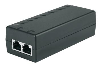
Use PoE Injector with PD (Powered Device) to expand your network connectivity to areas where there are no power outlets. The idea is to power up IP devices utilizing single ethernet cable providing data transfer & power supply.
